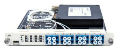
Light source unit is a stable light-emitting equipment. Inside use the DFB laser, its features is good light stability, high luminous power, long working life, etc. Output channel number can be customized, support luminous channels open or closed.
