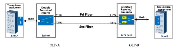
Note: the wavelength of PD1 and PD2 need to be specially customized, generally choose one of the SiteA wavelength as the monitoring wavelength.
