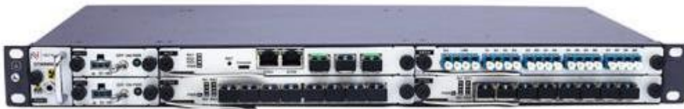
NS-DWDM-OP01 1U WDM Transmission System
